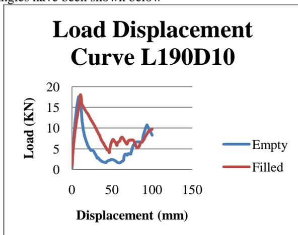
Load Displacement Curve for L/D=5 at 10°
