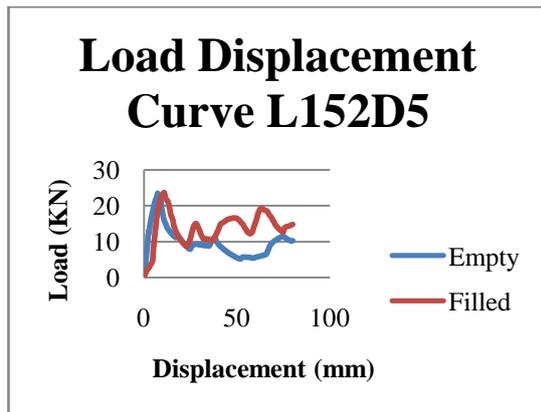
Load Displacement Curve for L/D=4 at 5°
