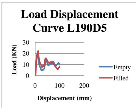
Load Displacement Curve for L/D=5 at 5°
