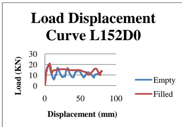
Load Displacement Curve for L/D=4 at 0°
