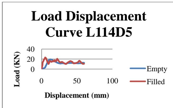
Load Displacement Curve for L/D=3 at 5°
