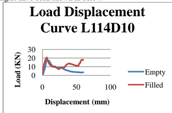
Load Displacement Curve for  $L/D=3$  at  $10^\circ$
