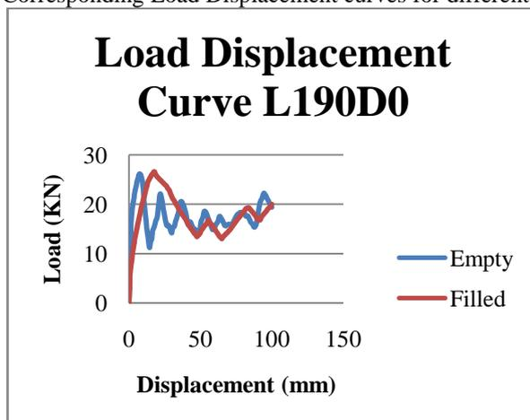
Load Displacement Curve for L/D=5 at 0°
